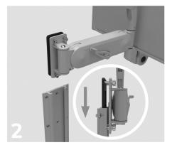
Insert MightyMount sliding bracket into track and loosely tighten 1/4" hex bolts at preferred mounting height.
