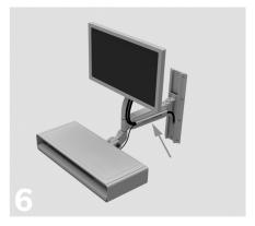
Attach display cables and thread cables through detacheable cable guard. Tie wraps may be inserted through hole in display neck for additional security.
