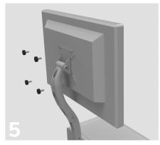
Use M4x8 or M4x12 thumb screws to attach display to display mounting bracket.
