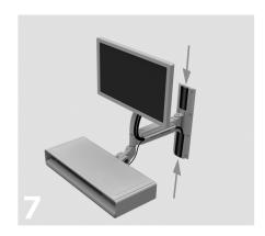
Trim supplied track cover to desired length and slide into mounting track channel as shown.
