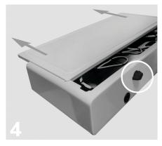
To access internal USB hub, twist rear latch 1/4 turn and slide keyboard enclosure top outward.
