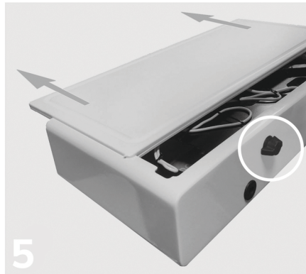
5 To access internal USB hub, twist rear latch 1/4 turn and slide keyboard enclosure top outward.
